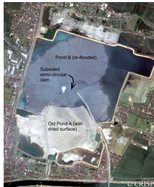
Figure 7: Satellite (IKONOS) photo (24.06.9) of the area flooded by the LUSI mud discharges.
